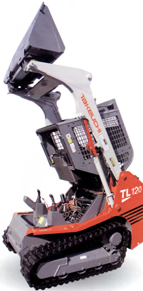
Tilt-Back Operator's Compartment for Easy Service Access
