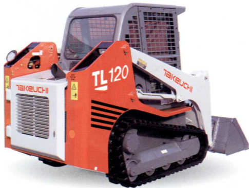
Track Undercarriage Provides Stable Work Platform
