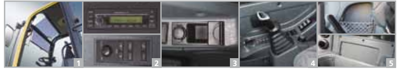
Roll-up Sun visor Radio / MP3-player with remote control Hands-free cell phone Ergonomic joysticks Storage compartments
